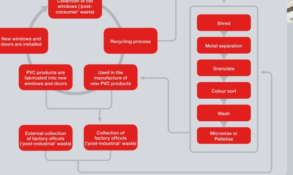
In 2017 we produced approximately 13.2k tonnes of recycled PVC compound for use in our extrusion processes. Of the recycled compound produced, 8.3k tonnes (being almost exclusively derived from post-consumer waste) was used alongside virgin resin in the manufacture of many of our rigid PVC products in our primary extrusion processes. This represents 17% of material consumption, up from 14% in 2016.
